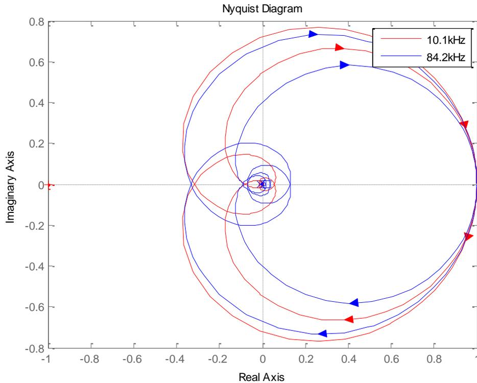
**Figure 3-19 Nyquist criteria of ITM showing improved stability with 2useconds delay**
