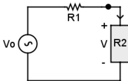
Figure 3-10 Voltage divider circuit
