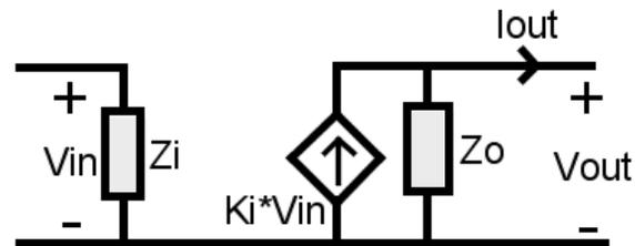
**Figure 2-4 Controlled Current Amplifier**
