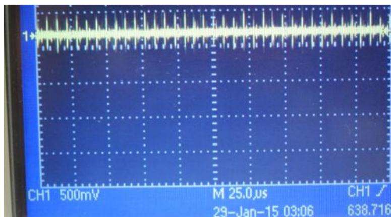
**Figure 3-4** Interface noise on voltage output channels
