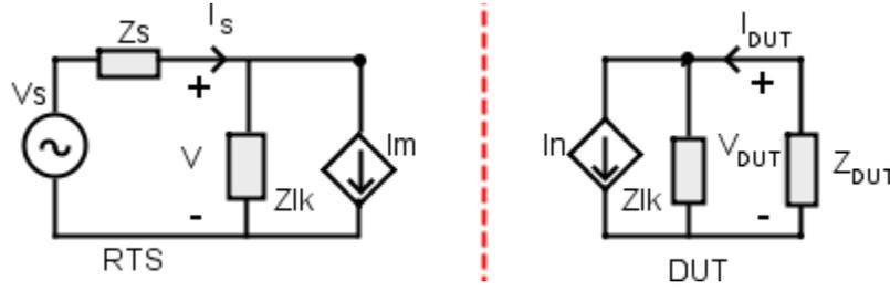
Figure 2-13 Transmission line method - Norton Equivalent
