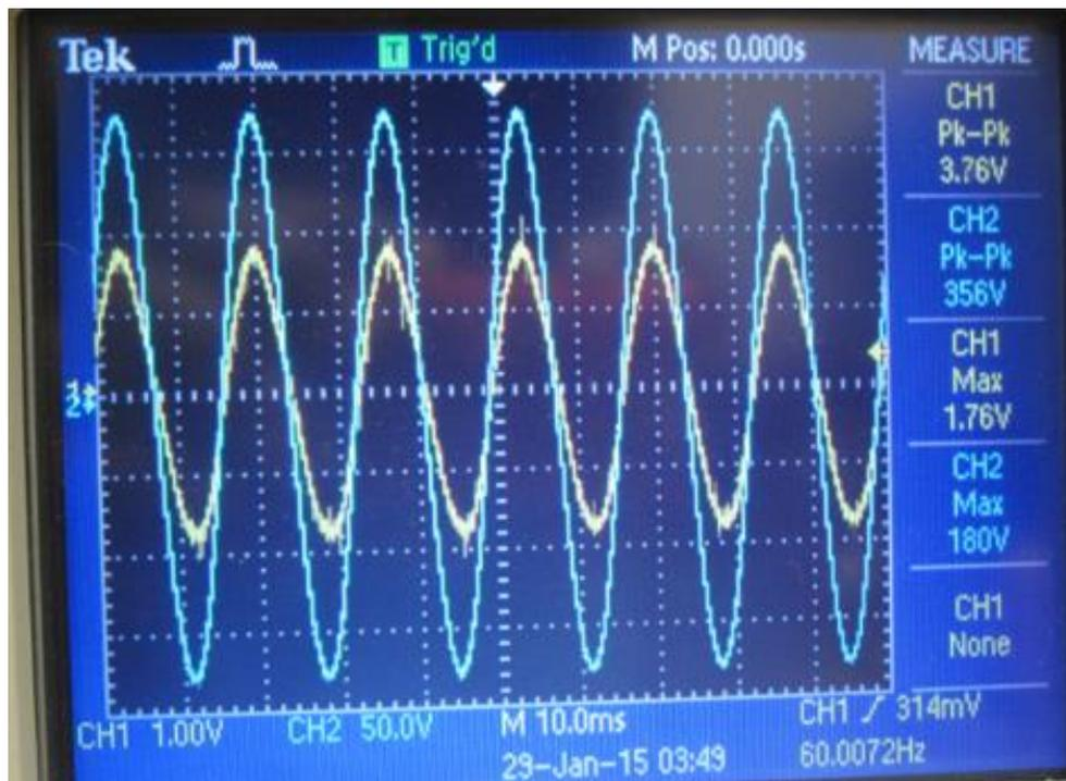
**Figure 3-5 Blue curve is amplified voltage signal, yellow curve is the voltage on the monitor channels.**
