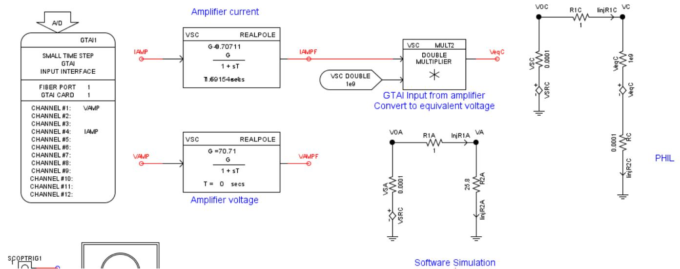
**Figure 3-20 PHIL interface of voltage divider in small time step**
