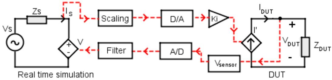
**Figure 2-9 Current Type: Ideal Transformer Method**
