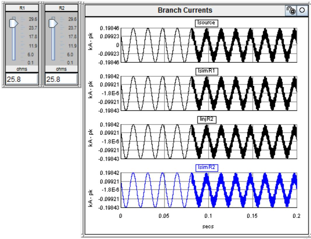
Figure 3-18 Software simulation of PHIL interface showing instability
