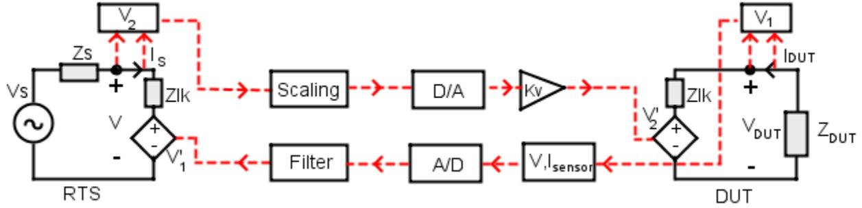
Figure 2-12 Transmission Line Method – Thevenin Equivalent
