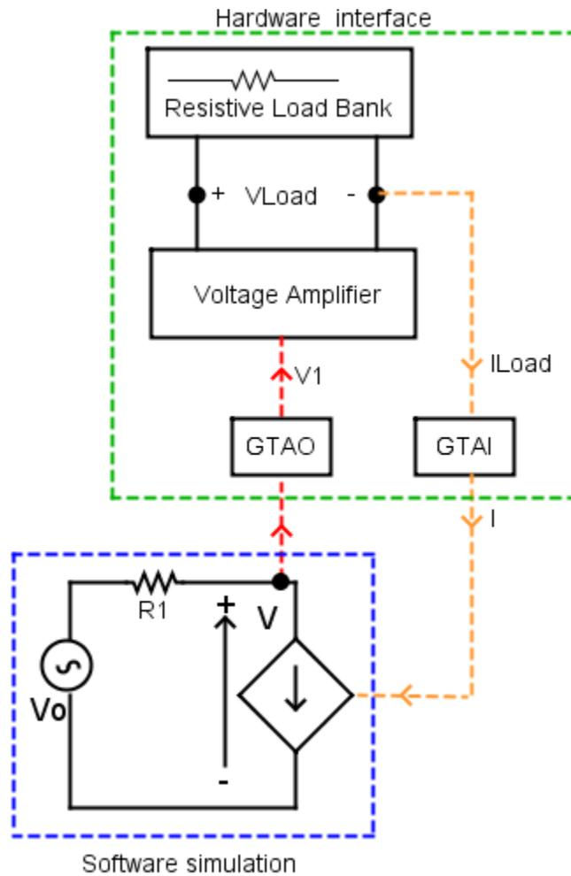
**Figure 3-11 Hardware-Software PHIL Ideal Transformer Interface**
