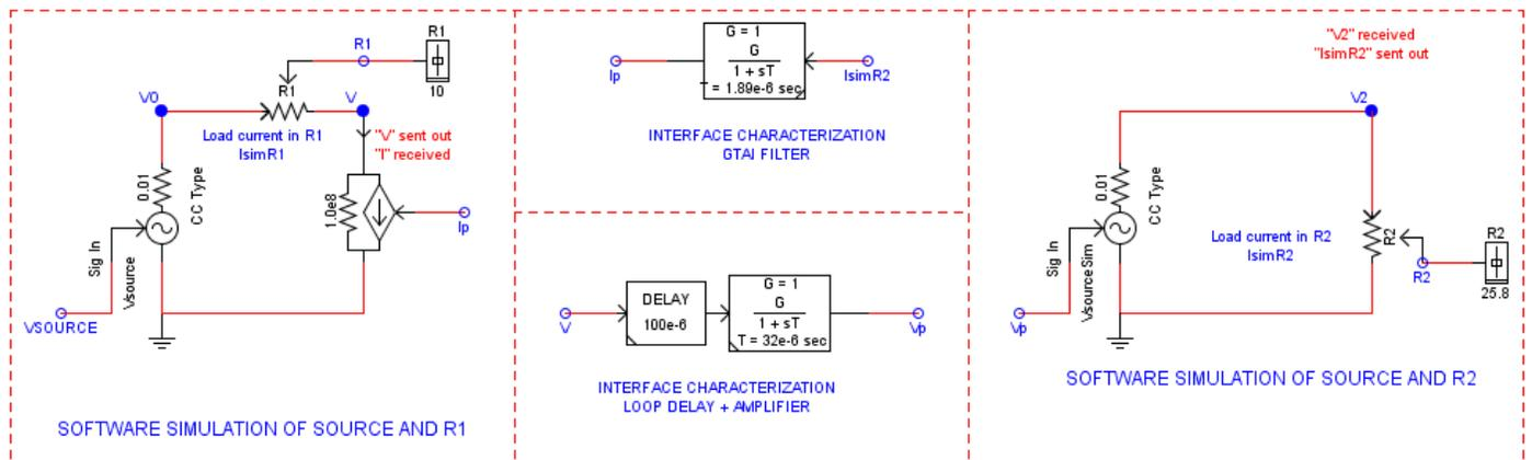
Figure 3-17 Software simulation of PHIL interface
