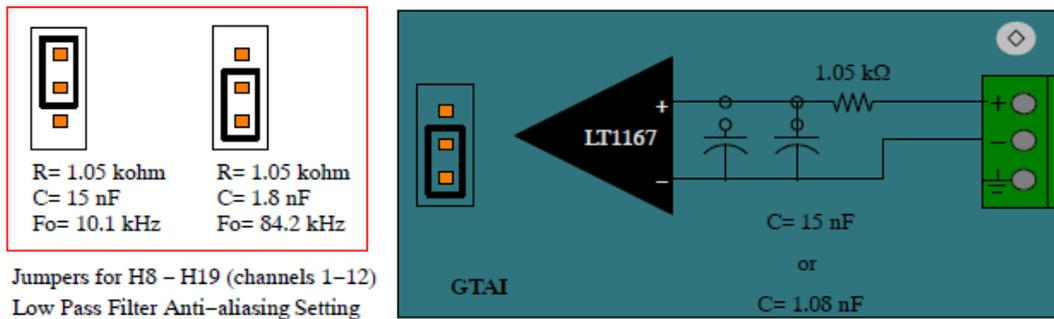
Figure 3-8 Anti-aliasing filter on GTAI channels
