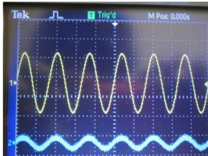
**Figure 3-3** Blue curve is the monitored amplifier monitor voltage channel, yellow curve is the GTA0 output sine wave applied to the amplifier's external input channels. Note the measurement ratio is 1V:100V
