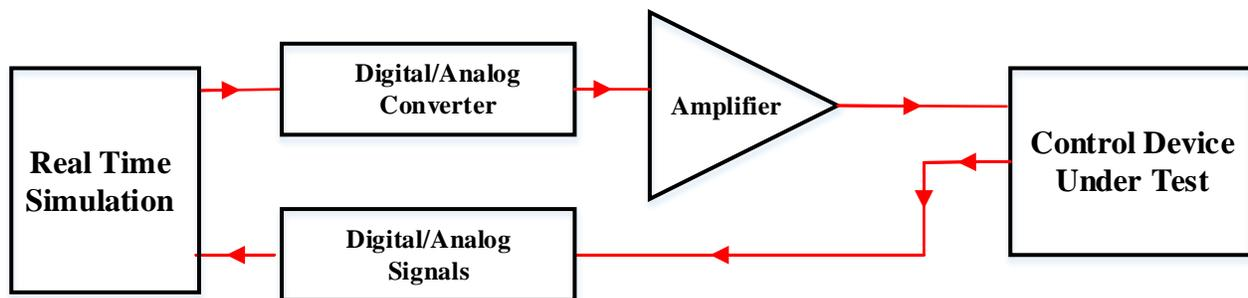
Figure 1-1 Control hardware in the loop simulations
