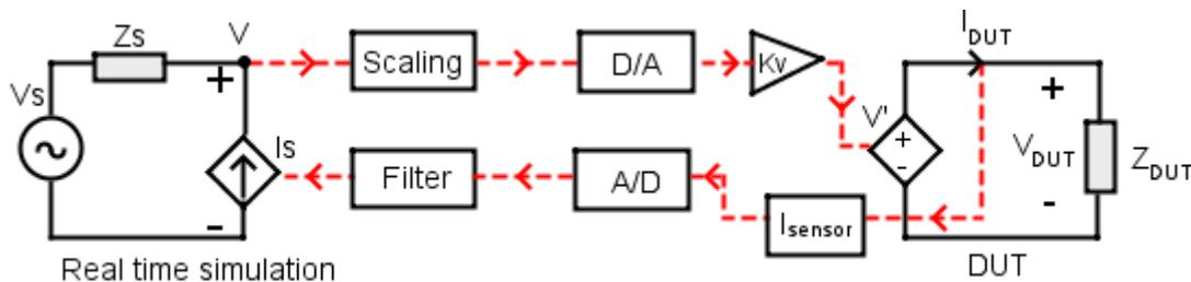
Figure 2-8 Voltage Type: Ideal Transformer Method
