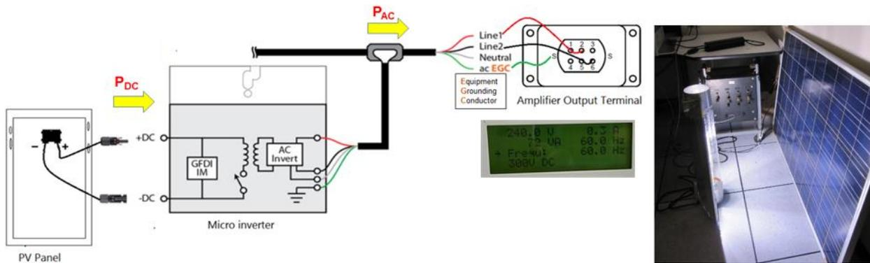
Figure 4-1 PHIL interface with PV Inverter
