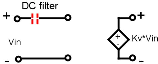
Figure 2-5 Filtering DC component from amplifier input
