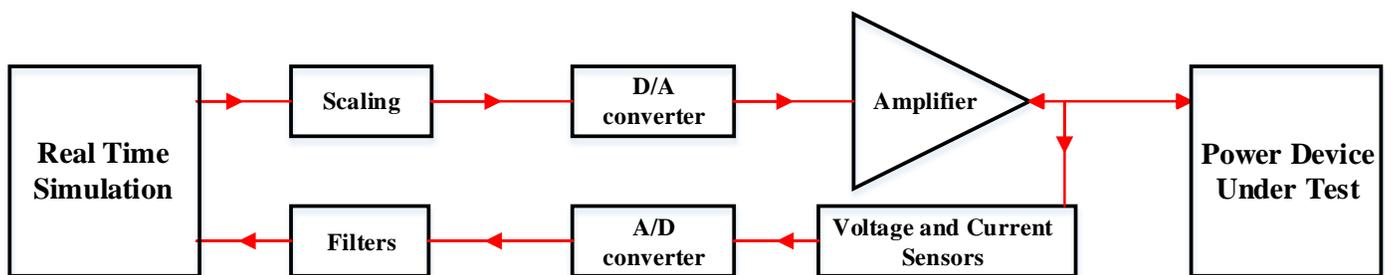
Figure 2-1 Power hardware in the loop simulations
