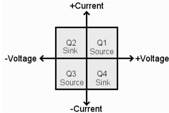
**Figure 2-2 Four quadrant amplifier operation for PHIL simulations**
