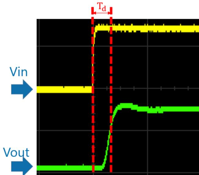
Figure 2-7 Step response to obtain amplifier transfer function characteristics
