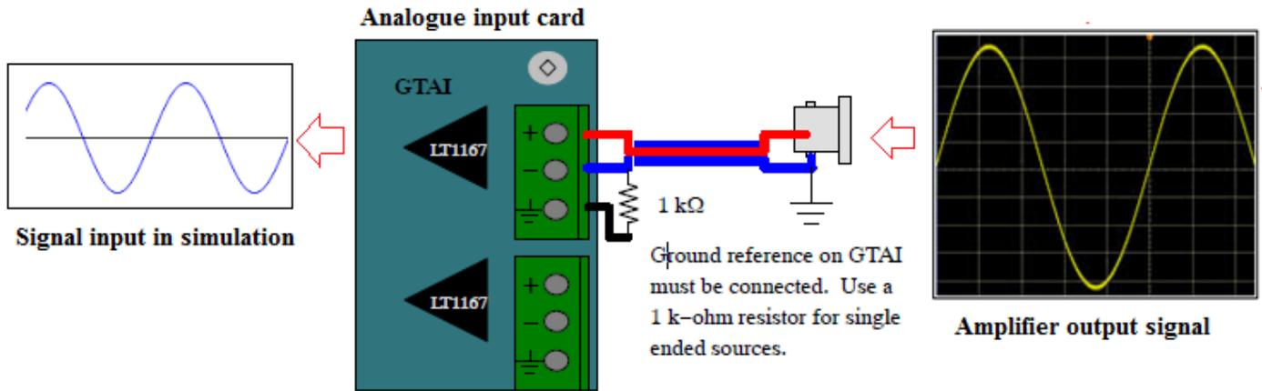
Figure 3-6 Amplifier output sent to simulation using GTAI card
