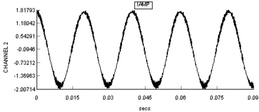
Figure 3-21 Unfiltered closed loop current signal from small DT GTAI channel
