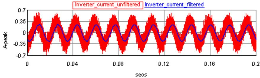
Figure 4-2 Inverter current in the RTDS
