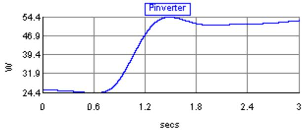
Figure 4-3 Inverter power observed in the RTS increases by 50% when filter cutoff is changed from 500Hz to 5kHz.
