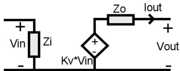
**Figure 2-3 Controlled Voltage Amplifier**
