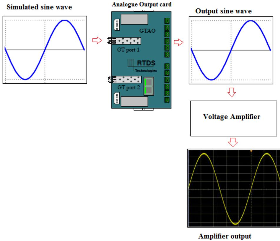
Figure 3-2 Amplifier gain testing
