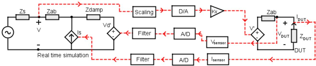
Figure 2-15 Damping Impedance Method
