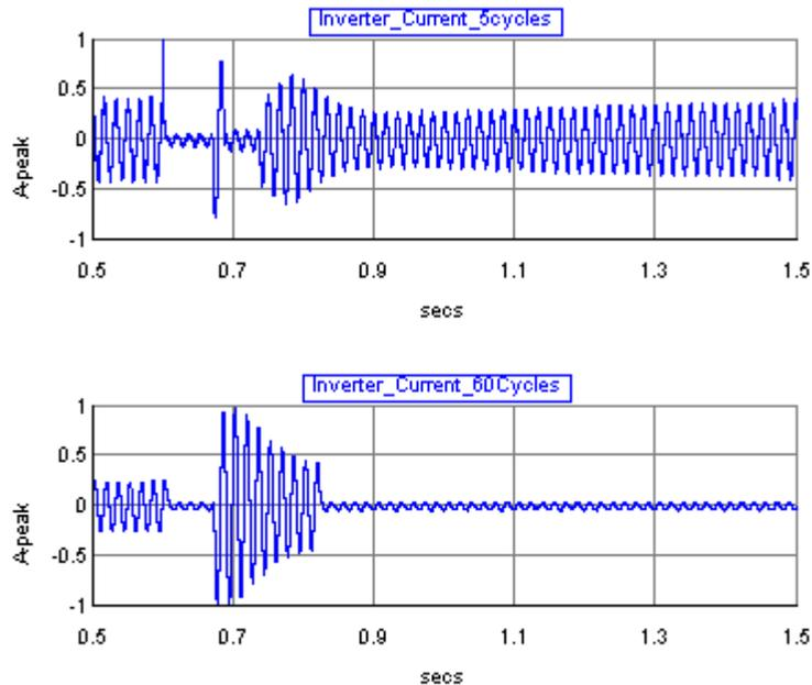
Figure 4-4 Inverter AC current response to a 5 cycle and 60 cycle, line to ground fault condition simulated in the RTS
